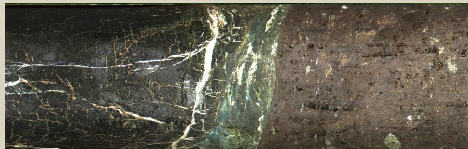
Figure 3: This is a cropped image of core G27 from the Southwest Deforming Zone. Note the transition from black shale, through sheared serpentine, into foliated fault gouge (left to right). (Zoback et al., 2011).
