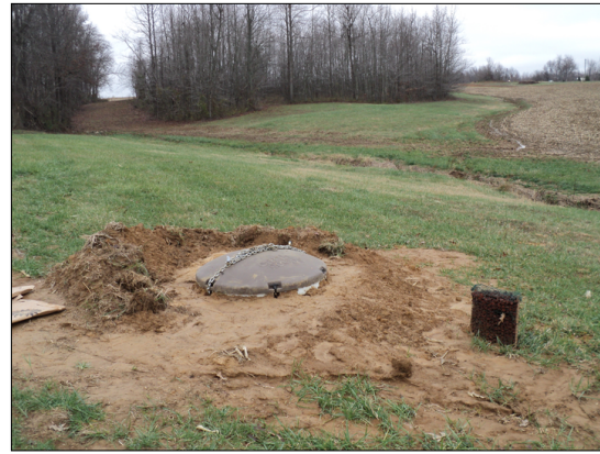
Figure 2: An atmospheric acoustic sensor package (enclosure in the lower right houses the ports for the high performance barometer and an infrasound microphone) installed at a Transportable Array station. The data from these sensors are openly distributed in the same manner as all Transportable Array data. (This work is in collaboration with an NSF MRI-R2 grant to the University of California, San Diego.)
